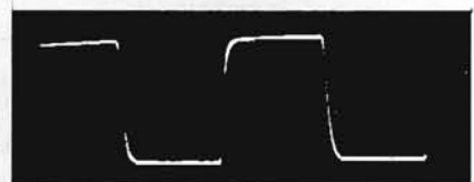
Fig. 11. 10 KC square wave from Dynakit (below) is much like original (above).
