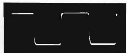
Fig. 11. 10 KC square wave from Dynakit (below) is much like original (above).
