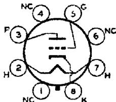
Glass-octal heater-cathode type used as rf power amplifier and oscillator. May be used with full input up to 30 Mc. For operation at 60 Mc, plate voltage and plate input should be reduced to 96 per cent of maximum ratings; at 90 Mc, to 98 per cent. Requires Octal socket and may be mounted in any position. OUTLINE 19, Outlines Section. Plate shows no color when tube is operated at maximum CCS ratings. The 1626 is used principally for renewal purposes.
