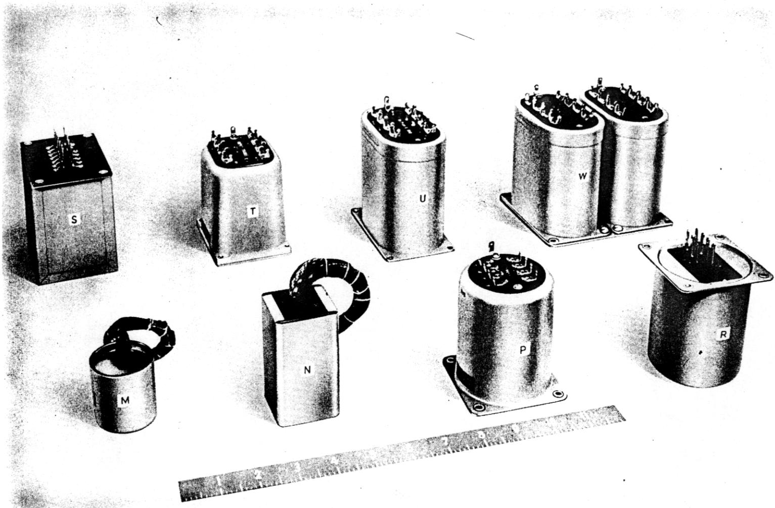
Fig. 2 Transmission Transformers M to W
